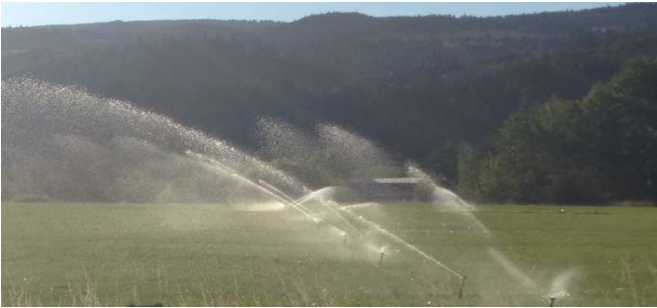
Impact sprinklers on handline
