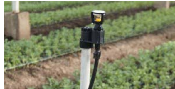
Solid set micro sprinkler
